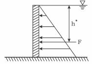
Moment of hydrostatic force about top edge of the gate
