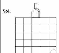
**Trash rack:** Is a metal frame provide in front portion of sluice gate of penstock to keep out debris and not to allow floating and suspended materials into penstock.
