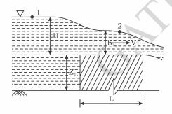
Q =  $C_d \times Area$  of flow  $\times Velocity$ =  $C_d \times (L \times h) \times \sqrt{2g(H - h)}$
