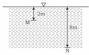
$$\frac{P_M}{P_N} = \frac{\gamma_W h_M}{\gamma_W h_N} = \frac{h_M}{h_N} = \frac{2}{8} = \frac{1}{4} = 1:4$$
