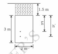
Centre of pressure  $h^* = \overline{h} + \frac{I_G}{A\overline{h}}$
