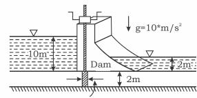
$$\begin{split} F_{\text{Net}} &= F_{\text{Left}} - F_{\text{Right}} \\ &= \rho.g. \; \overline{h}_1.A - \rho.g. \; \overline{h}_2.A \\ &= 1000 \times 10 \times \left(10 + \frac{2}{2}\right) \times \left(3 \times 2\right) - 1000 \times 10 \times \left(2 + \frac{2}{2}\right) \left(3 \times 2\right) \end{split}$$
