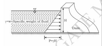
Total pressure on the vertical surface wetted per unit length = Area of the pressure diagram
