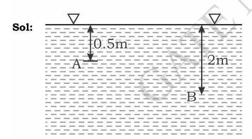
$$\frac{P_{A}}{P_{B}} = \frac{\gamma_{W} h_{A}}{\gamma_{W} h_{B}} = \frac{h_{A}}{h_{B}} = \frac{0.5}{2} = \frac{1}{4} = 1:4$$
