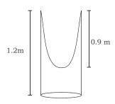
$$V_{\text{spilled out}} = V_{\text{paraboloid}}$$
