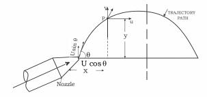
**Sol:** The total horizontal distance travelled by the fluid particle is called horizontal range of the jet, i.e. the horizontal
