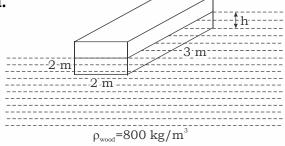
$$S_{\text{wood}} \times V_{\text{wood}} = S_{\text{water}} \times \overline{V}$$
