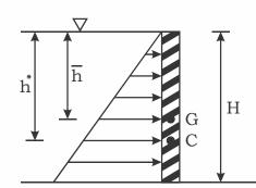
Depth of centre of pressure, h\* = centroid of pressure prism
