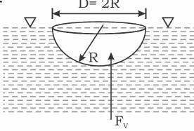
$F_v$  = Vertical component of hydrostatic force = weight of the fluid displaced by the body =  $\gamma v$
